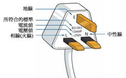
3-pin plugs must be marked with all the information as shown on the diagram.
